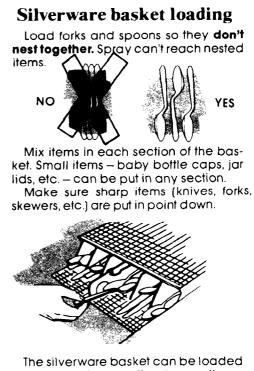
The silverware basket can be loaded while it's in place on the door, or it can be taken out for loading on the counter or table.
